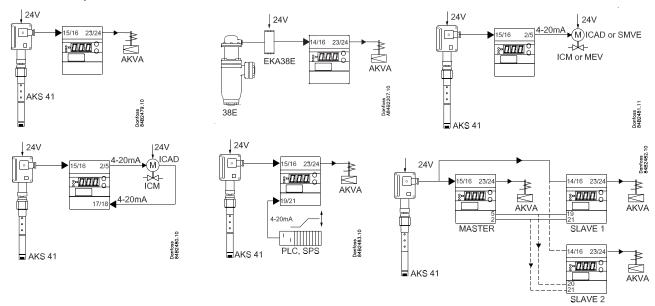
EKC 347 - ON/OFF Application. Open/Close solenoid valve with coil 110 V
